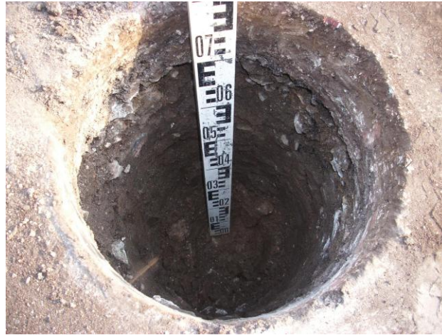
Schurf 3 ( Station 1+806), Steine/Packlager von 60-80 cm
