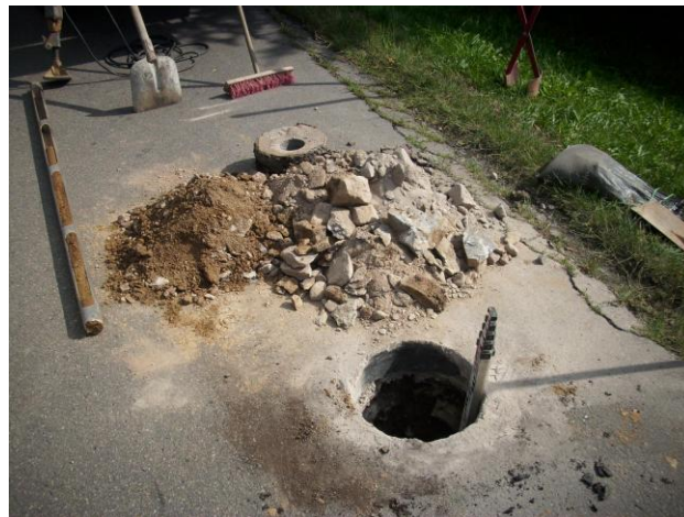
Schurf 7 (Station 2+215), Steine/Packlager von 55-70 cm
